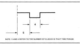
Figure 10. Asymmetrical Square-Wave Output Resulting from Count of 9
